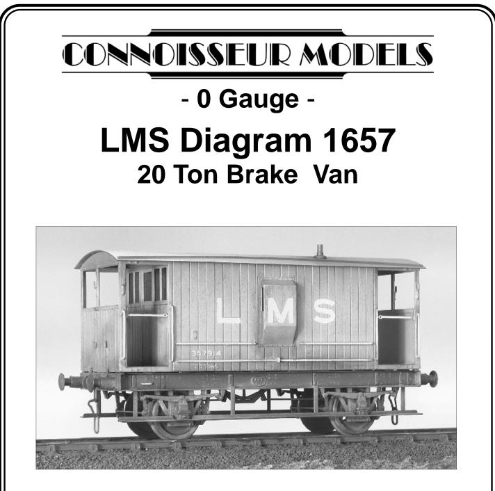
**Prototype.** 950 vehicles were built between 1927 and 1931 .They lasted well into BR days. As they got older and more Dilapidated extra strapping was applied and this is included in the kit .
